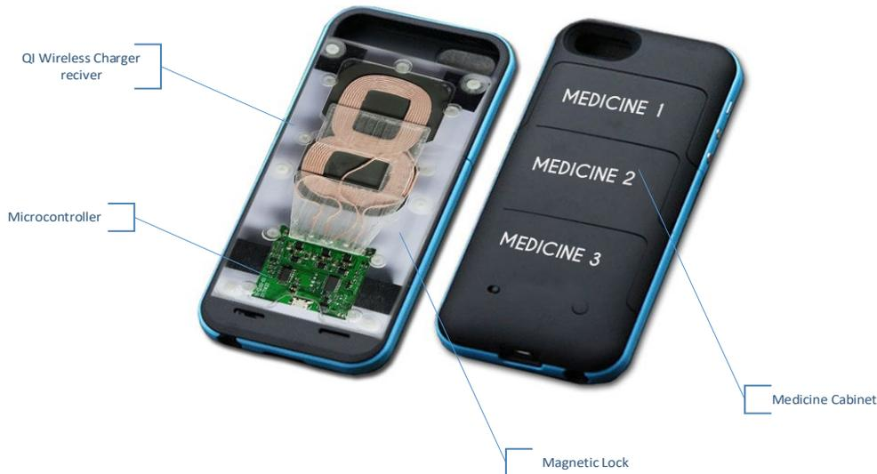
The data transaction between software application and the hardware is very low and thus, no battery is required, rather, QI coils (Li, 2016) are used to power the microcontroller to manage the communication and open the magnetic locks for each cabinet.
