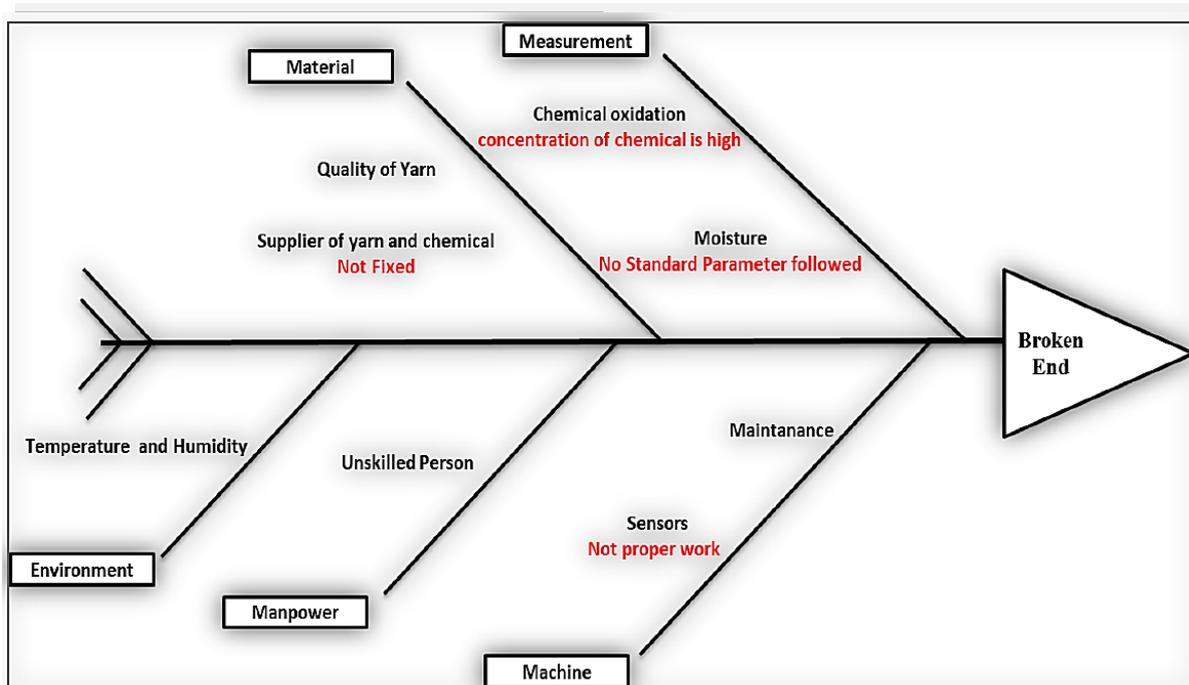
**Figure 3.** Cause and effect diagram of Broken End (BE)
