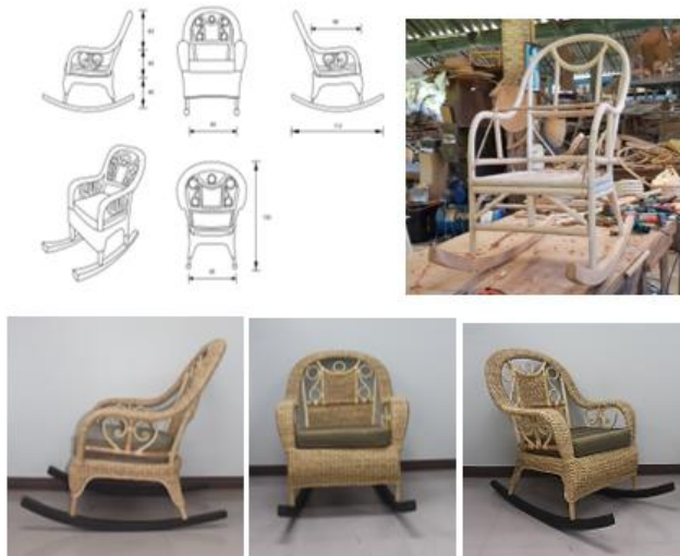
Figure 3 A sketch of rocking chair development. A drawing of chair structure made of rattan and real wood and wrap weaving with water hyacinth strips. The seat is with 10 cm. foam cushions for comfortable sitting, 2 armrests, 50 X 50 cm. wide in size, 45 cm high from floor to seat, 120 cm high from floor to backrest, and 112 cm long of the base rocking wood
