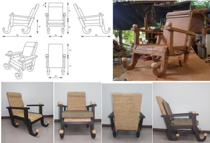
Figure 5 A sketch of easy chair development. A drawing of chair structure made of real wood and wrap weaving with water hyacinth strips. The seat is with 10 cm. foam cushions for comfortable sitting, 2 armrests, 50 X 50 cm. wide in size, 40 cm high from floor to seat, 120 cm high from floor to backrest, adjusted declining degree, decorated with 6 lathed wood in ball-shape of 8 cm in diameter as an extra advantage for user's hand and foot massage to relax muscles.
