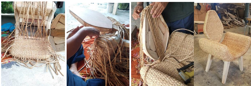
Figure 2 Weaving process for water hyacinth furniture started with the armrest, the backrest, to complete every side of the chair
