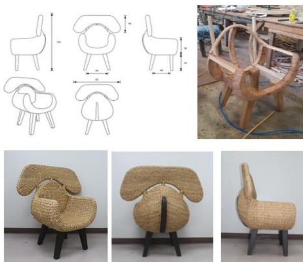
Figure 4 A sketch of easy chair development. A drawing of chair structure made of real wood and wrap weaving with water hyacinth strips. The seat is with 5 cm. foam cushions for comfortable sitting, 2 armrests, 40 X 40 cm. wide in size, 40 cm high from floor to seat, and 120 cm high from floor to backrest.
