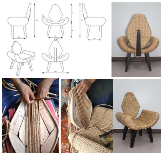
Figure 6 A sketch of easy chair development. A drawing of chair structure made of real wood and wrap weaving with water hyacinth strips. The seat is with 5 cm. foam cushions for comfortable sitting, 2 armrests, 40 X 40 cm. wide in size, 40 cm high from floor to seat, and 87 cm high from floor to backrest. cm.
